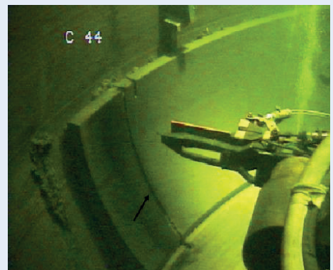
Manipulator with CAMC tool at Karlsruhe Multi Purpose Research Reactor
