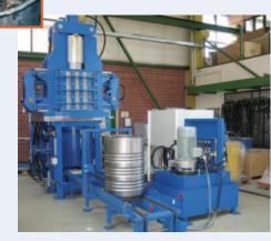
Effective compaction of filter elements, Ignalina nuclear power plant (Lithuania)
